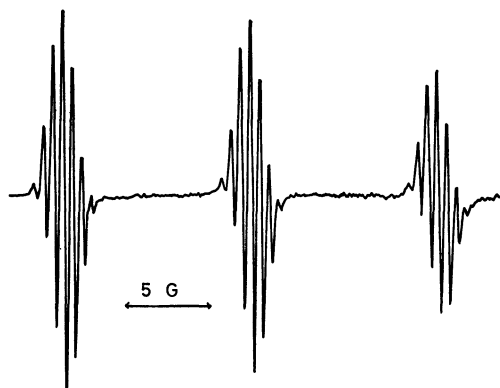
Fig. 4. The ESR spectrum of 3,3',5,5'-tetrachlorodibenzenesulfenamidyl radical ( 2r ) in benzene at room temperature.
